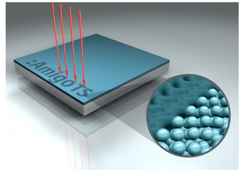
Infra-red energy from 830nm laser diodes exposes the image area. During this process the thermoplastic pearls absorb the heat energy and melt, forming an insoluble resin that is firmly bonded to the aluminium substrate. Unexposed areas remain unhardened and are easily removed with the Clean Out Solution. This physical imaging process is referred to as ThermoFuse™ technology.
